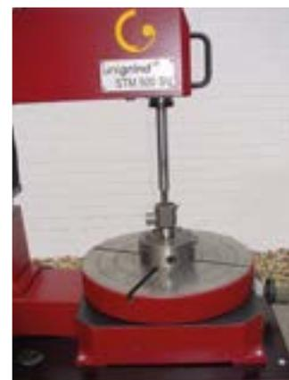
Grinding safety relief valve on rotary table
