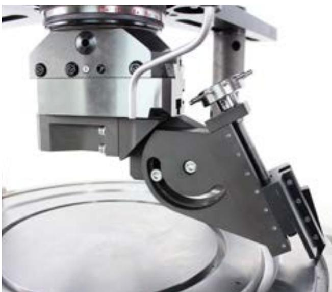
FDA 500, RTJ 'V' grooves machining
