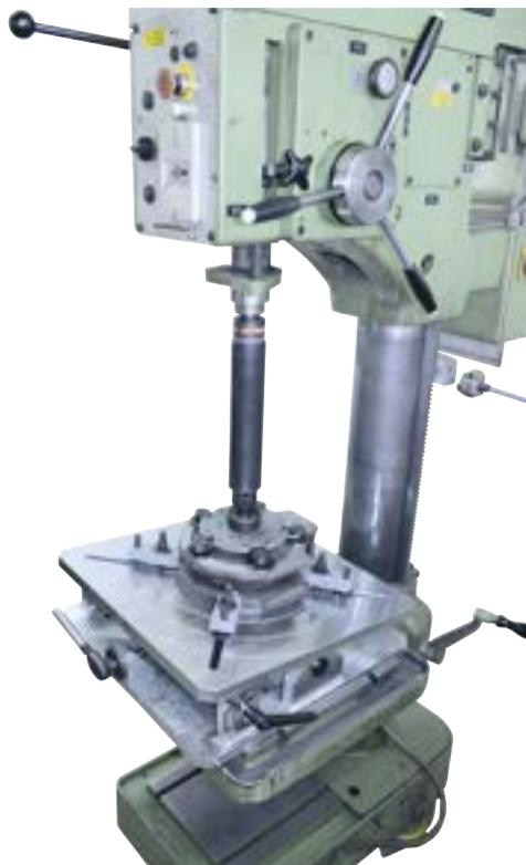
UNT 2 + Adapter, Grinding gate valve wedge
