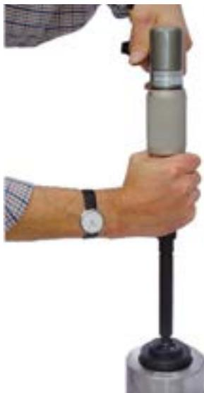
KVS-Lens Grinding sealing surface
