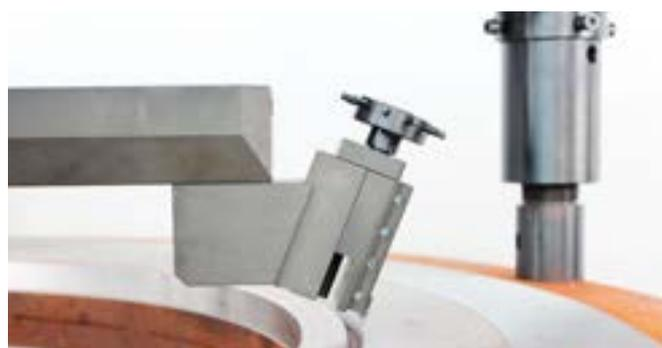
FDA 1200, RTJ 'V' grooves machining
