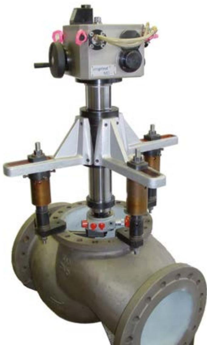
MD 1 Machining of globe valve seat
