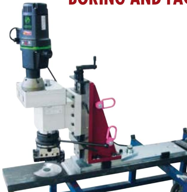
Mobile boring and turning machine for all boring and turning operations during steel work.
