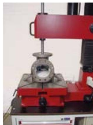
Grinding gate valve on tilting table
