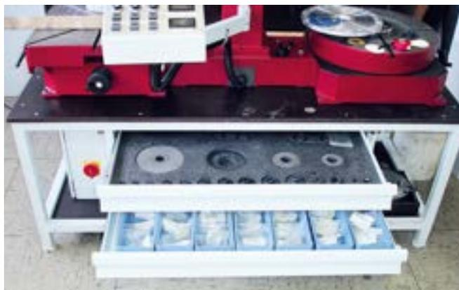
**Stationary valve grinding and lapping machine for sealing surfaces in gate, globe, check valves, gate valve wedges and safety relief valves.**
