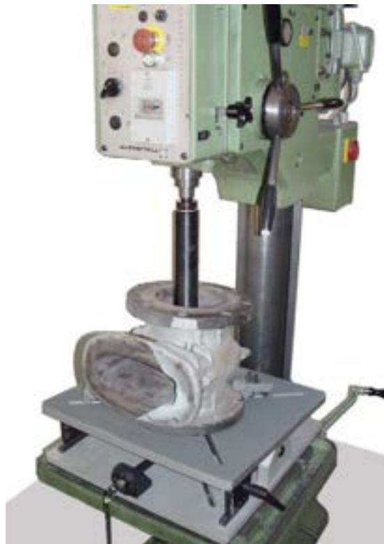
UNT 2 + Adapter, Grinding gate valve seat
